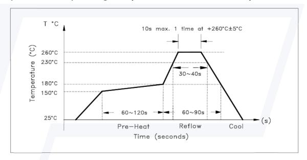
This reflow profile is applicable for RoHs compliance with exempt and Non-Pb free parts. (Low temperature Sn-Pb conventional solder.)
