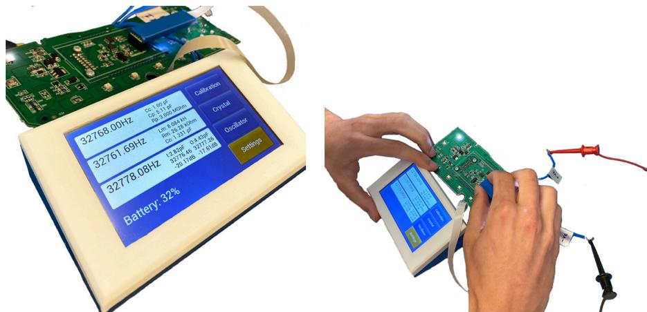
Design engineers often optimize their circuit performance via trial and error, at the expense of significant investment in time. Measurements to verify the performance become increasingly sensitive if the timing loop utilizes a tuning fork (32.768kHz) crystal. These crystals are extremely sensitive to loading effects and extreme care and accuracy is essential to determine the in-circuit behavior of these components.
