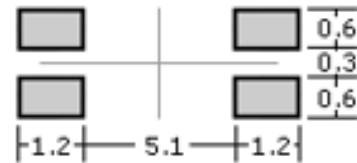
Figure 2) Land Pattern - Top View
