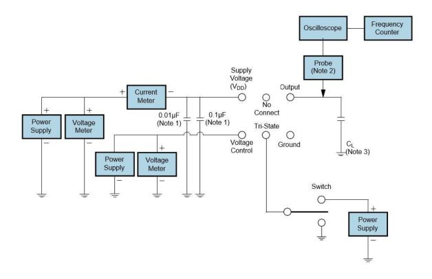
Note 1: An external 0.01µF ceramic bypass capacitor in parallel with a 0.1µF high frequency ceramic bypass capacitor close (less Than 2mm) to the package ground and supply voltage pin is required.
