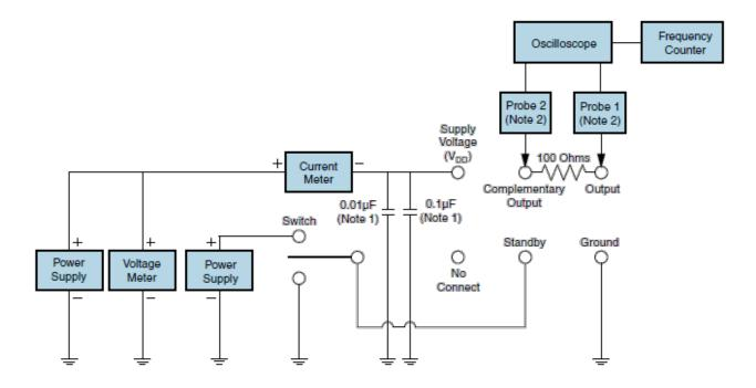
Note 1: An external 0.01µF ceramic bypass capacitor in parallel with a 0.1µF high frequency ceramic bypass capacitor close to (Less than 2mm) the package ground and supply voltage pin is required.
