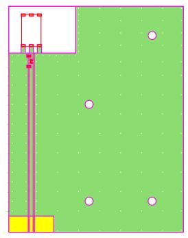
Dimension: 54mm\*70mm Substrate material: FR4 dielectric constant: 4.4 Copper thickness: 35um Copper layer: 2 Stacking information: Copper\_35um/FR4\_730um\_/Copper\_35um Data: 2023.08.10
