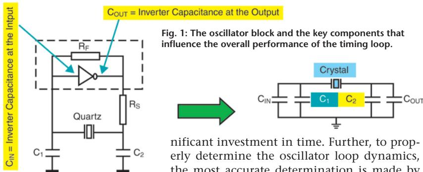
Fig. 1: The oscillator block and the key components that influence the overall performance of the timing loop.
